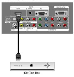
Note: When the Set Top Box output is DVI signal, then the Audio cable should be connected.
